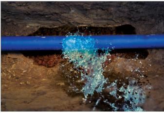
Typical longitudinal crack in a pipe typicaly caused by earth settlement or increased traffic load.
